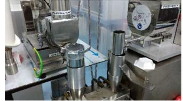
Micro-extruder (10g/batch), mini-extruder 1 kg/h...
