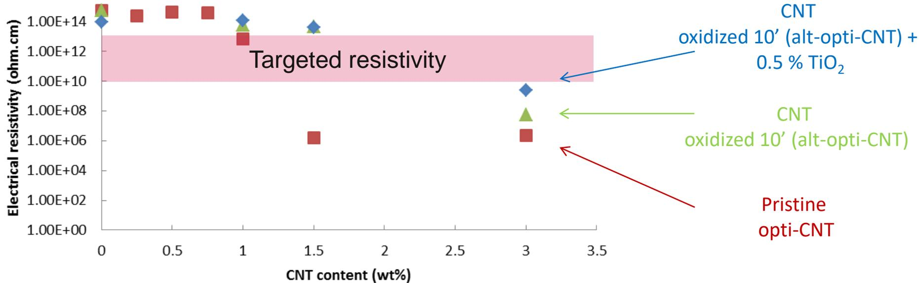
Percolation threshold can be tailored with oxidation of CNT and adding TiO<sub>2</sub>
