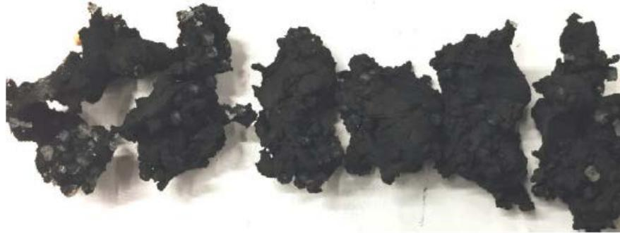
**m-ETFE/ETFE/opti-CNT impossible to dilute during the compounding stage
