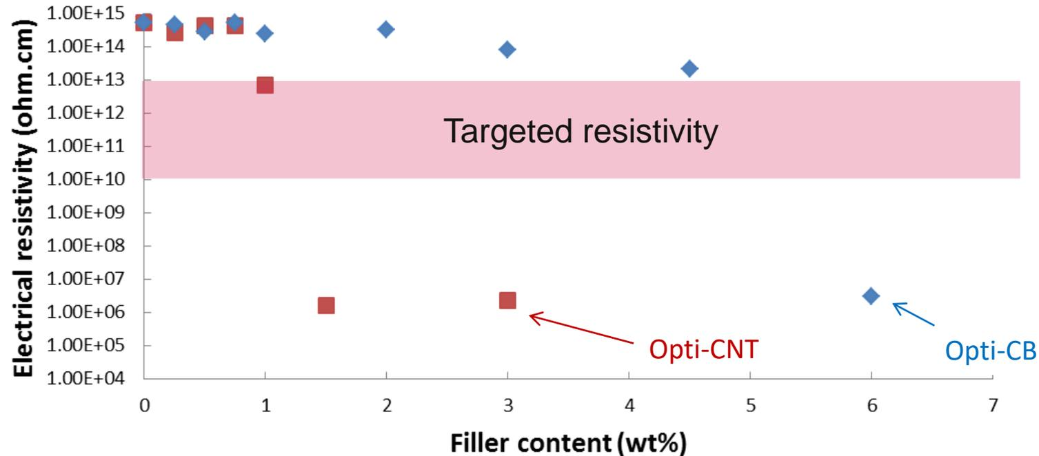
**CB provides a softer percolation threshold compared to CNT**
