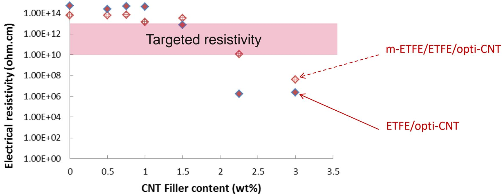
Percolation threshold can be tailored by mixing ETFE with a chemically modified ETFE → **ETFE/m-ETFE/opti-CNT (50/50/1.875) selected**
